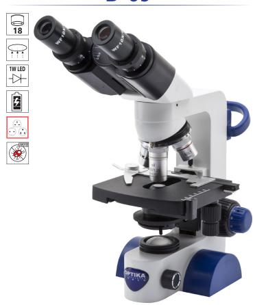
Cordless, modern binocular microscope ideal for students and mainly primary schools with achromatic lenses (1000x), FN 18 eyepieces, finite optical system, coaxial focusing, StagErase™ eraseable mechanical stage, Abbe condenser and 1 W LED illumination with rechargeable batteries. Slim and easy to carry, it is equipped with arm/wrist rest support to reduce the fatigue during use and long lasting LED illumination to provide over 20 years of use
