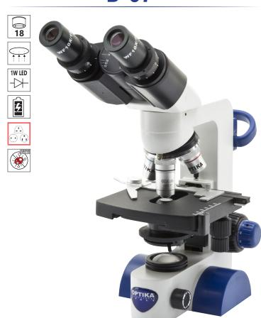
Cordless, modern binocular microscope ideal for students and mainly primary schools with achromatic lenses (600x), FN 18 eyepieces, finite optical system, coaxial focusing, StagErase™ eraseable mechanical stage, Abbe condenser and 1 W LED illumination with rechargeable batteries. Slim and easy to carry, it is equipped with arm/wrist rest support to reduce the fatigue during use and long lasting LED illumination to provide over 20 years of use
